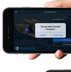
Important: when checking for update, make sure that your mobile device has Internet connection and the optical device is not connected to mobile device.
