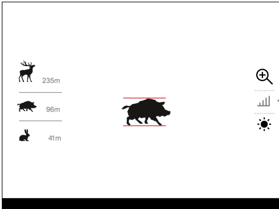
1. Select the **Stadiametric Rangefinder** function with short presses of the **M (9)** button until the icon
