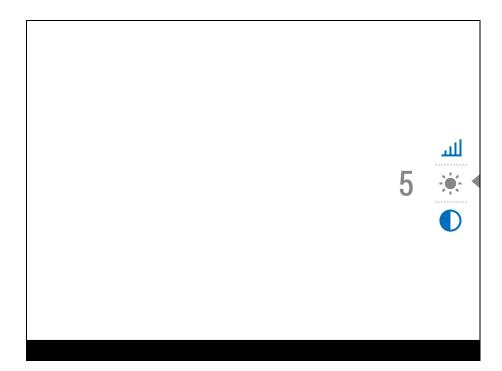
**Brightness** - press the **UP (10)** / **DOWN (8)** buttons to change display brightness from 0 to 20.
